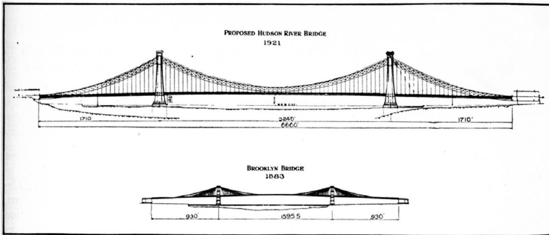
Figure 4. Elevation of proposed Hudson River Suspension Bridge compared with that of Brooklyn Bridge (Scientific American, 1921a)
