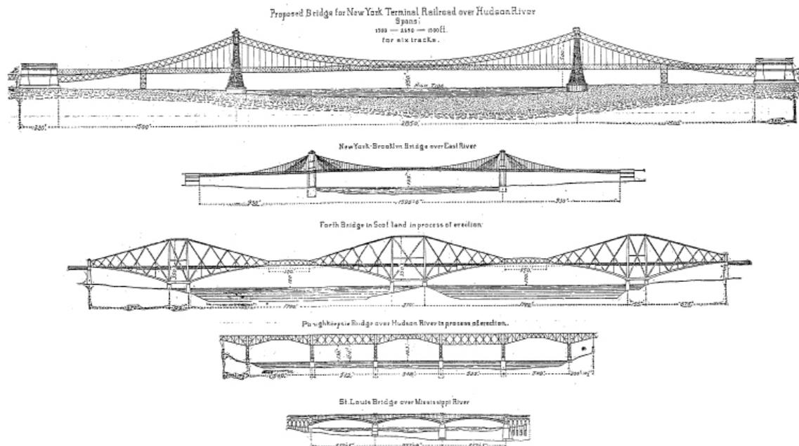
Figure 2. The proposed elevation of the Hudson River bridge (top) compared to already constructed bridges (Engineering & Building Record 1888a)
