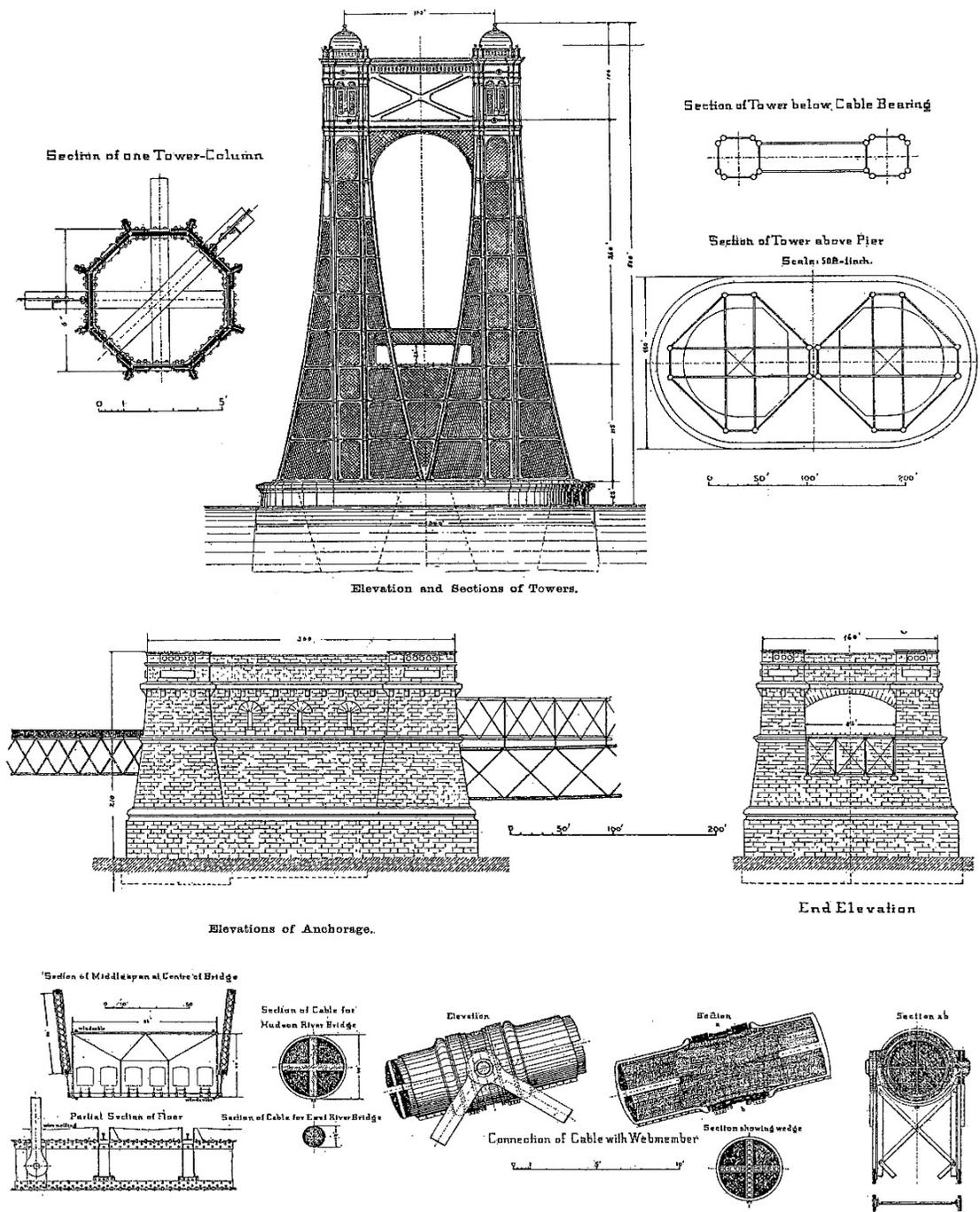
Figure 1. Details of the railway suspension bridge across the Hudson River proposed by Lindenthal in 1888 (Engineering News, 1888a)
