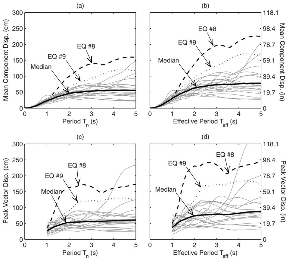
**Fig. 11.** Spectral displacement for 16% damping for individual records in the 2/50 year event: (a) and (b) mean of  $x$  and  $y$ -component displacement for a linear system and a bilinear system with given equivalent linear properties, respectively; (c) and (d) peak displacement in any direction for a linear system and a bilinear isolation system with given equivalent linear properties, respectively
