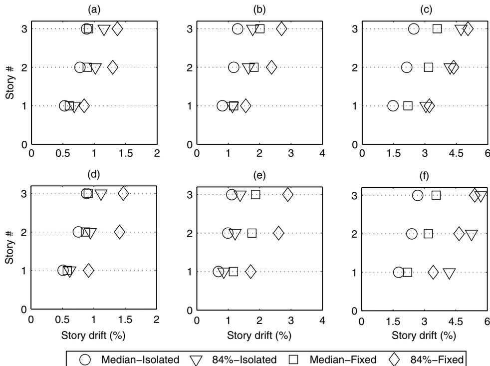
**Fig. 7.** Story drift ratio demands for: (a)–(c) 50/50, 10/50, and 2/50 year events, respectively, in  $x$ -direction; (d)–(f) 50/50, 10/50, and 2/50 year events, respectively, in  $y$ -direction
