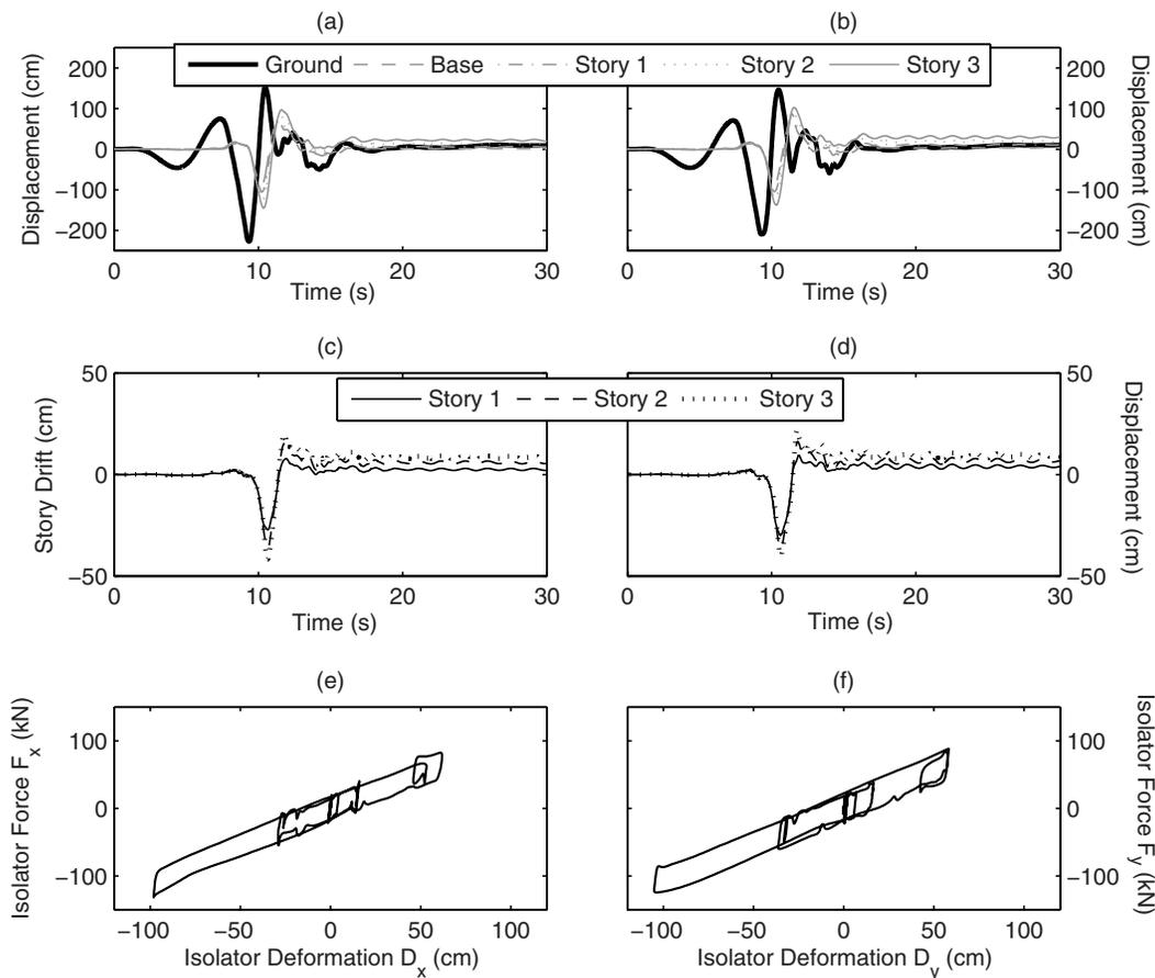
**Fig. 12.** History of IMRF responses to earthquake record #8: (a), (b) displacements at CM in  $x$  and  $y$ -directions, respectively; (c), (d) story drifts at top left corner in  $x$  and  $y$ -directions, respectively; (e), (f) top left corner isolator force-deformation in  $x$  and  $y$ -directions, respectively
