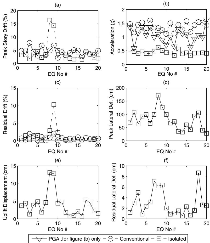
**Fig. 10.** (a) Peak story drift (%); (b) PGA and roof acceleration; (c) maximum residual story drift; (d) peak isolator deformation; (e) peak isolator uplift; (f) maximum residual isolator deformation sampled for individual motions in the 2/50 year event
