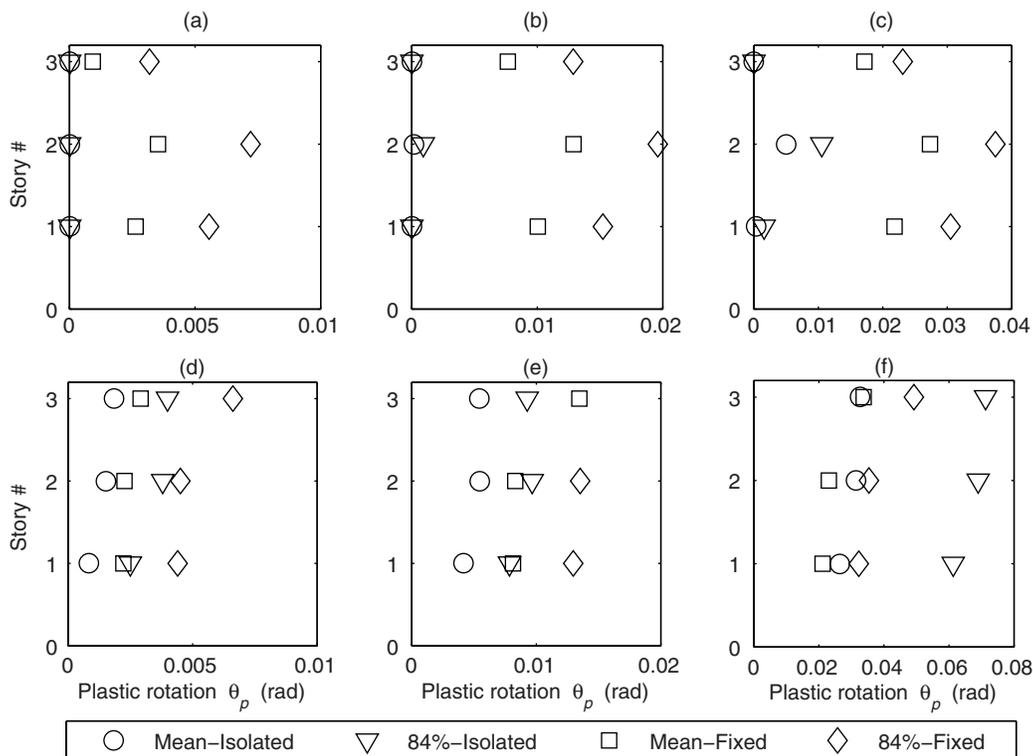
**Fig. 9.** Beam plastic rotation demands for: (a) 50/50; (b) 10/50; (c) 2/50 year events; and panel zone plastic rotation demands for: (d) 50/50; (e) 10/50; (f) 2/50 year events
