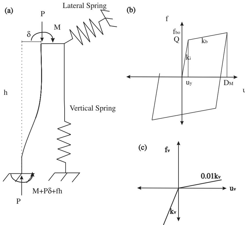
**Fig. 4.** (a) Isolator model composed of an elastic column element in parallel with lateral and vertical springs; (b) lateral force-deformation; (c) vertical force-deformation in the isolation devices
