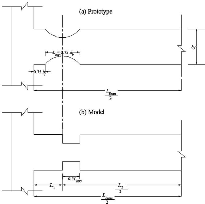
**Fig. 3.** (a) Plan view with typical geometry for RBS; (b) 3-element frame model;  $b_f$  = width of flanges and  $d_b$  = beam depth (not shown in plan view)
