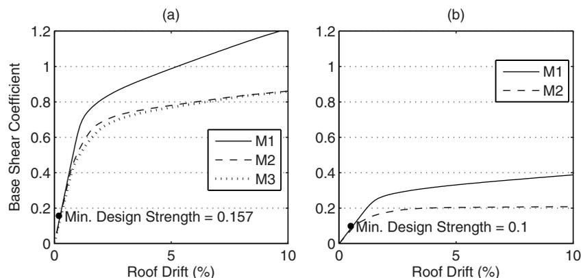
**Fig. 5.** Capacity curve: (a) conventional building; (b) base-isolated building, with design strength indicated
