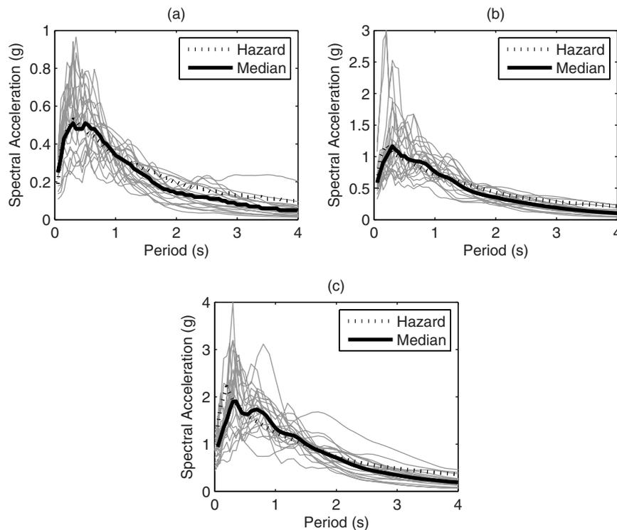
**Fig. 6.** Acceleration spectra for individual scaled motions, along with median and target spectra: (a) 50/50; (b) 10/50; (c) 2/50 year earthquake scenarios
