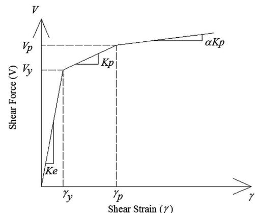
**Fig. 2.** Panel zone force-deformation behavior
