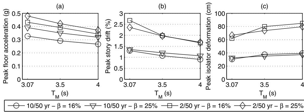
**Fig. 13.** Median values of: (a) peak floor acceleration; (b) peak interstory drift; (c) peak isolator deformation as a function of isolation system parameters in the 10/50 and 2/50 year events
